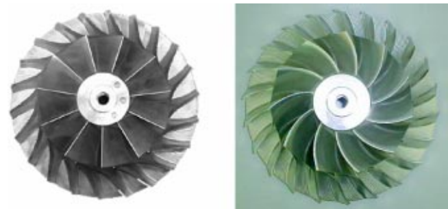
Fig. 3 Investigated impeller. Left: conventional E7X design. Right: inverse INV design.
