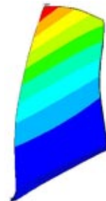
Fig. 7 Mode shape for unsteady TURBO-AE simulations
